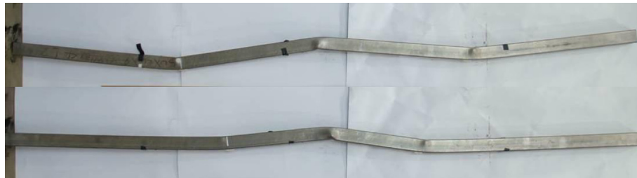
Fig. 14. Failure modes of SHS 50 × 50 × 3-1 – configuration: 1/2 span (top) and SHS 50 × 50 × 3-2 – configuration: 1/3 span (bottom).
