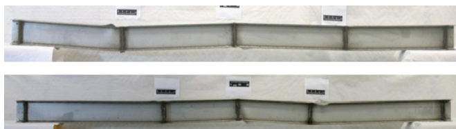
Fig. 15. Typical failure modes of I-200 × 140 × 6 × 6-1 – configuration: 1/2 span (top) and I-200 × 140 × 8 × 6-2 – configuration: 1/3 span (bottom).
