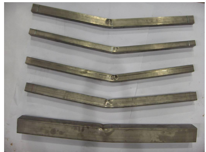
Fig. 4. Failure modes for simply supported RHS and SHS beams (from top to bottom: RHS 60 × 40 × 3-MA, RHS 60 × 40 × 3-MI, SHS 50 × 50 × 3, SHS 60 × 60 × 3, SHS 100 × 100 × 3).
