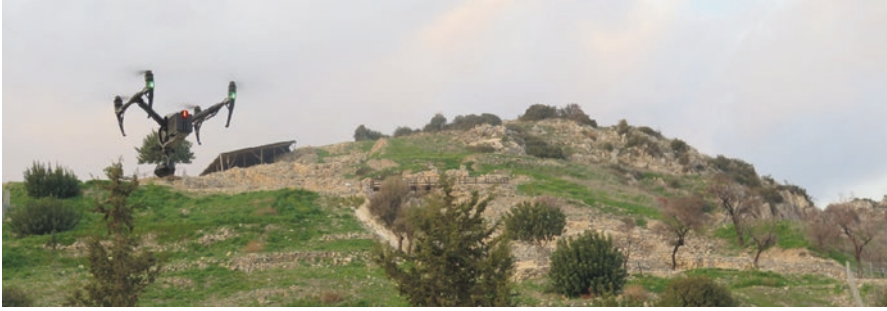
Fig. 24 Inspire 2 UAV with 20mp Zennuse X5S camera and sensors
