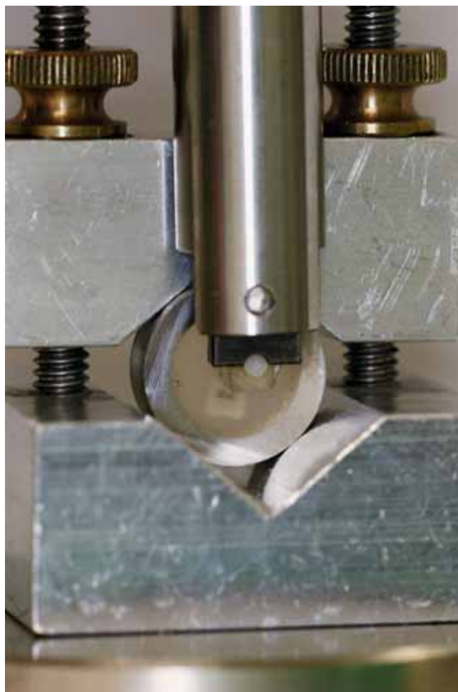
Fig. 1b The notched blade half encloses the composite cylinder and shears it off. The universal testing machine registers the fracture and thereby measures the bond strength.
