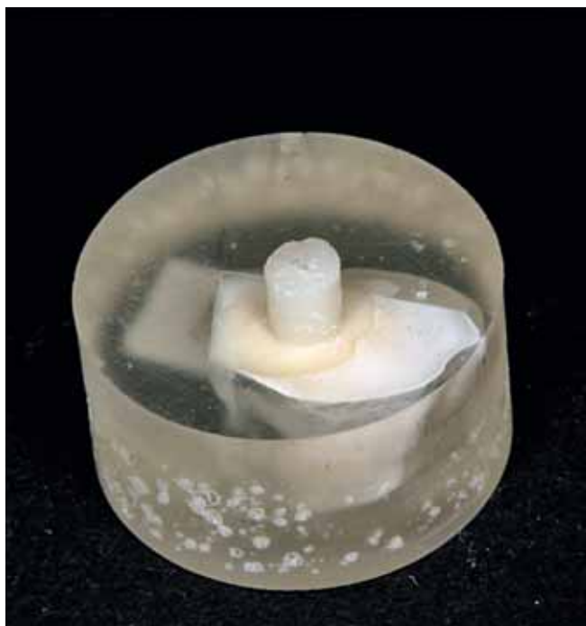
Fig. 1a Specimen for measuring shear bond strength. A composite cylinder made in a standardized mold is luted to the dentin surface.
